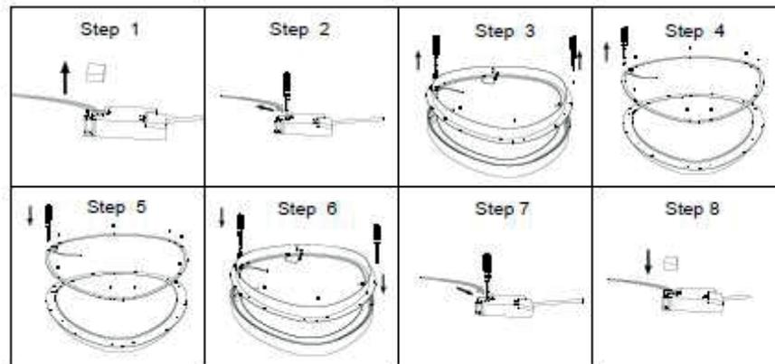
Step 1: Open the driver cover at the near end of the lamp - by hand.
